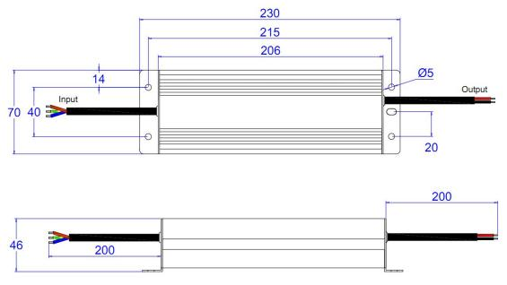
Input black(L) and white(N) wires to be connected to AC input, Green wire to be connected ground; output red and black wires to be connected to led lighting.
